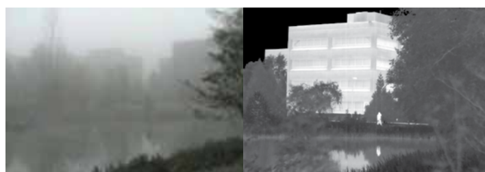
Thermal energy passes through many obscurants including smoke, dust, modest foliage and light fog. In this case the fog obscures this person from the regular CCTV camera, but on the thermal image the person shows up quite clearly.
