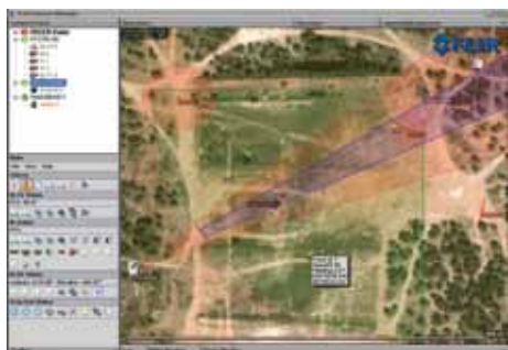
With the built in geo-mapping feature of the FLIR Sensors Manager software geo-calibrated sensors can be displayed on the map so that the operator can quickly assess the situation.
